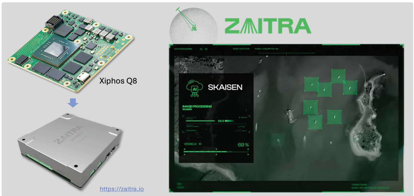
Figure 5: Example application where an AI/ML model is on-orbit and hosted on an FPGA (Credit: Zaitra )
